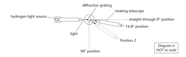
a. The lines on a diffraction grating are spaced 1.68 × 10<sup>-6</sup> m apart.
