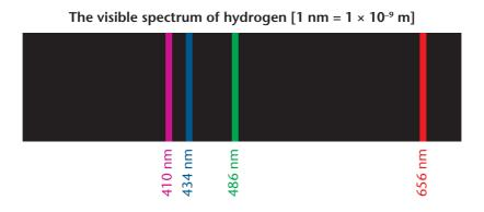
Light from a hydrogen source can be passed through a diffraction grating to form an interference pattern. The wavelength of each spectral line can then be determined by measuring the angle to its first order maximum.
