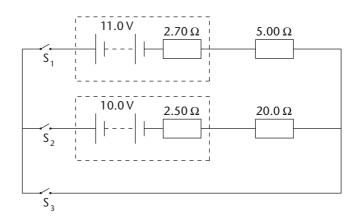
a. Switches  $S_1$  and  $S_2$  are closed and switch  $S_3$  is left open. Show that the current in the circuit is 0.0331 A.
