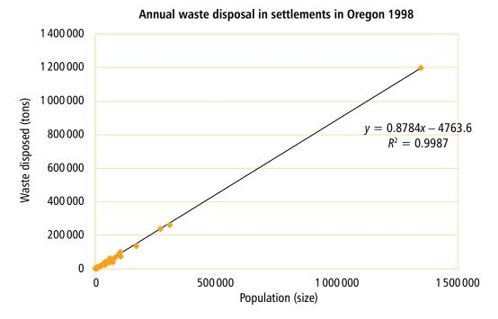
On your scatter graph you should have a line passing through the points, its equation (y = 0.8784x - 4763.6) and the coefficient of determination value  $R^2 = 0.9987$ .
