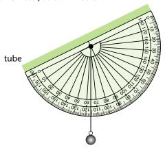
The thin tube should be fastened firmly to the diameter of the protractor for greater accuracy in sighting an object. It may be helpful to place a hair-line cross at the end of the tube to line up the object
