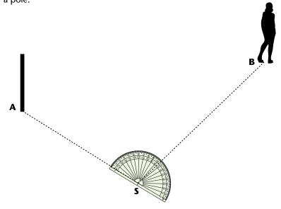
Keeping the angle measurer fixed on the stool, turn the needle and tube until another object B, say a student, is sighted. Record the reading in degrees on the scale.
