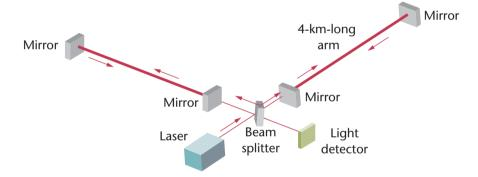
**b.** LIGO tunnels are kept at an ultra-high vacuum, which contains almost no particles. The beam splitter, which is made of glass, reflects half the light and transmits half the light, as shown below.
