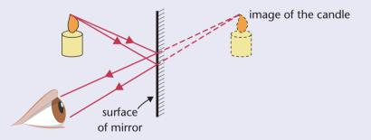
The image that is seen in a plane (flat) surface is the *same size* as the object and is the *same distance* behind the mirror as the object is in front of the mirror (image distance = object distance).
