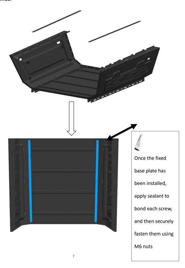
**Step 4: Install front and rear door frames**
