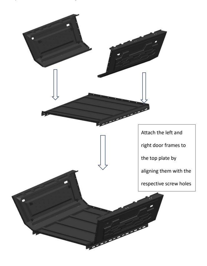
Step 3: Install the fixed base plate above the left and right door frames.
