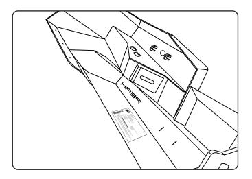
Ix Compliance plate on the passenger side bottom panel inside the bull bar. Note serial number and keep for your records.
