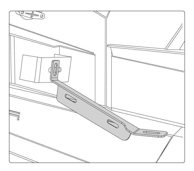
8. Install 2x M6 Cage nuts in centre for number plate bracket. Affix base plate of number plate bracket to bar using 2x M6 bolts.
