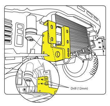
5. Begin by temporarily mounting the chassis brackets using the front two bolts and lower chassis mount point. Mark the locations for the rear bolt holes. Then, remove the chassis bracket and drill holes of 12mm diameter in preparation for the final installation of the chassis bracket and recovery point.
