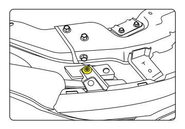
**4.** Affix grill using 2x domed plastic retainer screw pins sourced from original parts bin.
