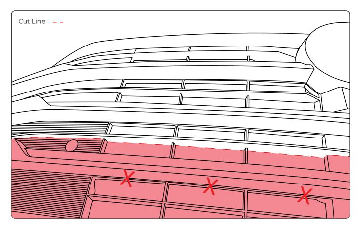
15. Cut grill along cut line with air hacksaw and clean up all cut edges.
