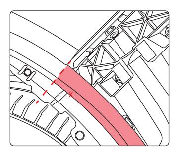
**16.** Tape up plastic wheel arch garnish and trim flush with the end of the quarter panel.
