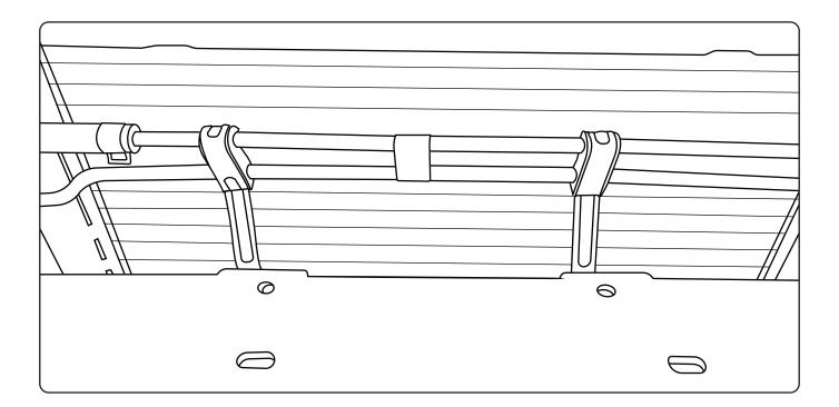
**10.** With the help of another person slide the bar onto the chassis mount and install 3x M12x40mm bolts, washer and nuts per side to hold the bar in place (pictures below).
