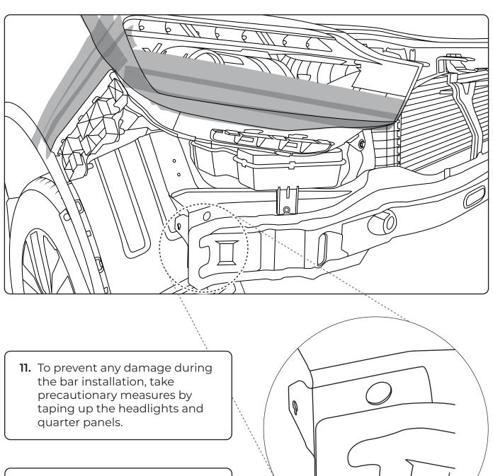
**12.** Trim body panel as per photo and cover exposed areas with epoxy based rust resistant paint.
