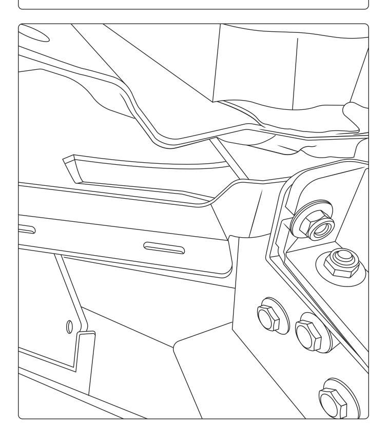
**14.** Enlist the assistance of another individual to securely fasten the three bash plates, beginning at the rear and progressing forward (Bash Plate 03, Bash Plate 02, Bash Plate 01), utilizing the M8x30mm bolts and washers.
