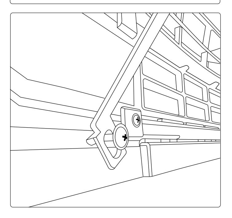
**13.** Mount the other side of wing support bracket to chassis mount using 1x M10x40mm bolts washers & nuts.
