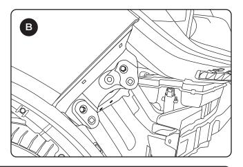
8. Using a Phillips head screwdriver remove plastic bumper retaining brackets from the quarter panels on both sides.
