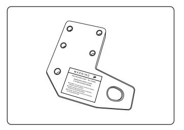
2x recovery point warning labels on the outer side of each recovery point.
