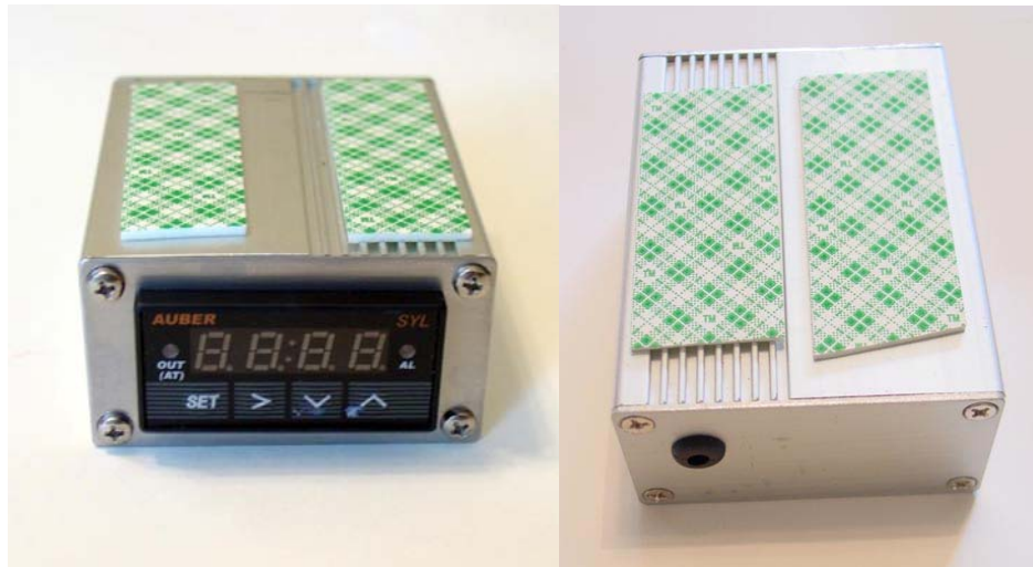
Figure 1. PID Controller, Aluminum extrusion box, rubber grommet, double sided tape pre-assembled - Front view on left. Back view on right.
