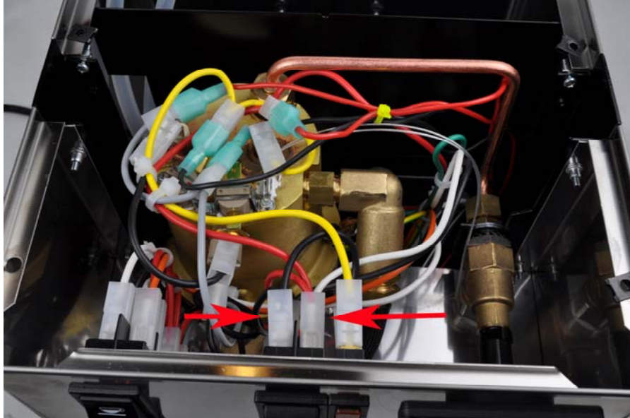
Figure 23a. Red arrow indicates the connectors that controller power cable will be tapped.
