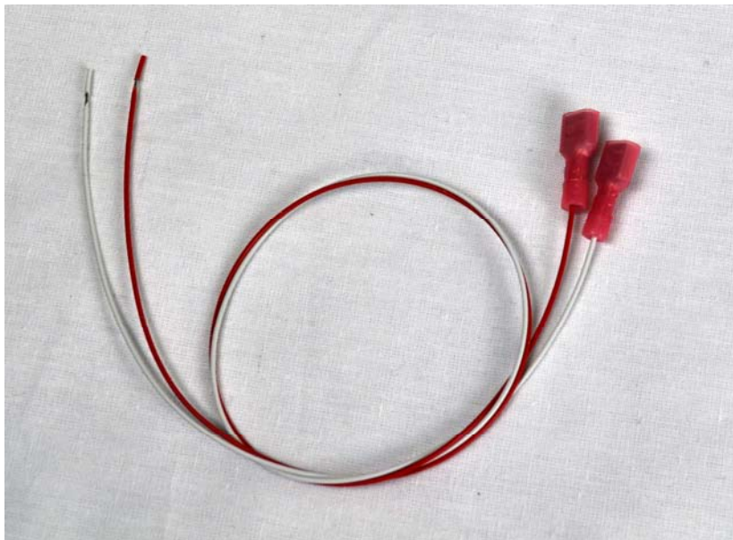
Figure 5. Cables for connecting controller brew control output to SSR brew control input. Red cable is for positive. White cable is for negative. They are terminated with female disconnect terminal on one end.
