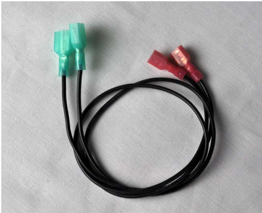
Figure 4. Pair of black cables for connecting SSR output to the cables that used to be on the steam thermostat. They are terminated with female disconnect on end and male disconnect on the other.
