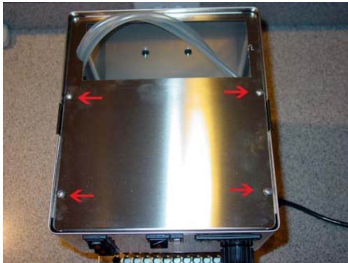
Figure 13. Top panel. Red arrows indicate the screws that hold the top panel.
