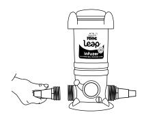
Attach the filter section of flex hose to one hose adapter and the return section of flex hose to the other hose adapter with clamps and tighten with screwdriver. Bi-flow valve design allows water flow installation in either direction.
