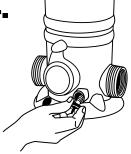
Unscrew knob from the front of FROG Leap Infuzer. Allow all water to drain.
