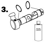
Replace both O-rings. Apply silicone lubricant that came with your FROG Leap Infuzer on O-rings.
