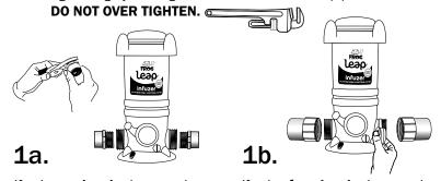
If using **male adapters**, apply pipe thread tape or sealant to the threaded end of each adapter.
