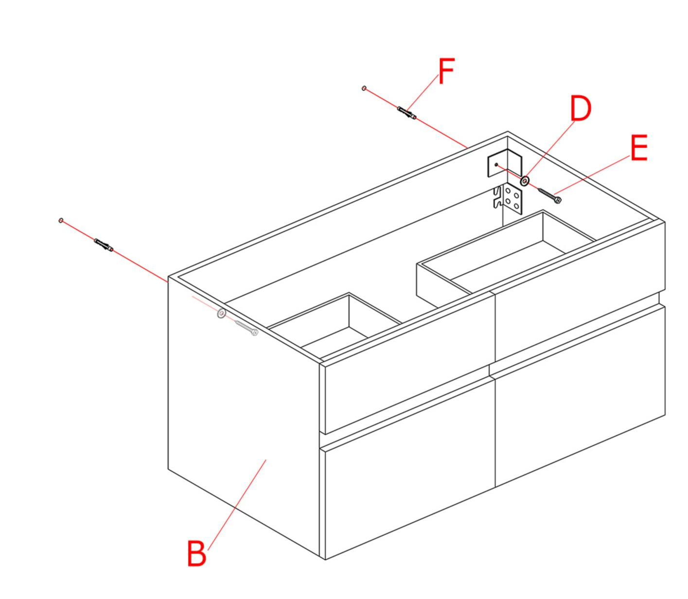
1. Put the cabinet body(B) to the wall and adjust the body to make sure that it is straight and level. According to the holes on the hinges at the corners of the body, mark to drill holes on the wall. Suit the expansion bolts(F) into the drilled holes and tighten the expansion screws(E) through the washers(D) and the holes on the hinges into the bolts in the wall as shown.
