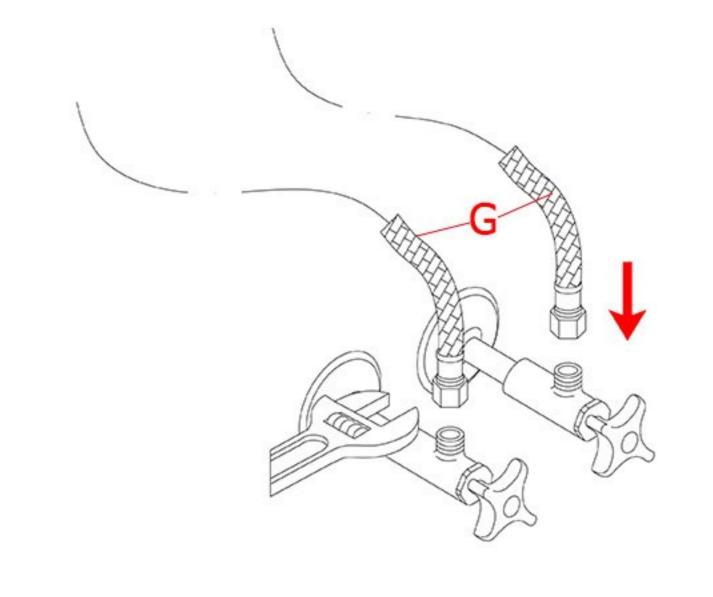
Screw up the waterlines (G) to the corresponding water supply outlets with adjustable wrench (not included).
