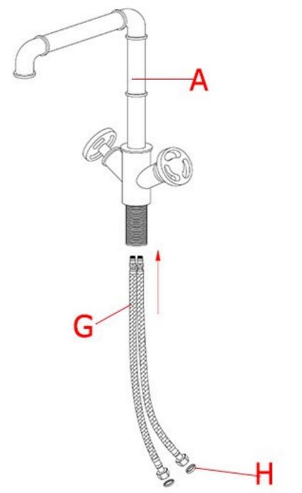
2. Screw up the cold/hot waterlines (G) to the corresponding holes under the bottom of the faucet body (A). Insert the spacers (H) to the other ends of the cold/hot waterlines (G).
