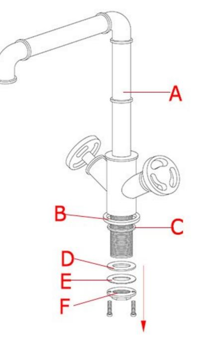
Remove the rubber washer (D), metal washer (E) and mounting nut (F) from the threaded pipe (B) and fit the decor washer (B) and O-ring (C) to the bottom of the faucet body (A).
