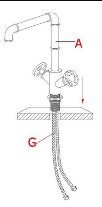
Insert the faucet body (A) and the waterlines (G) into the hole on the countertop.
