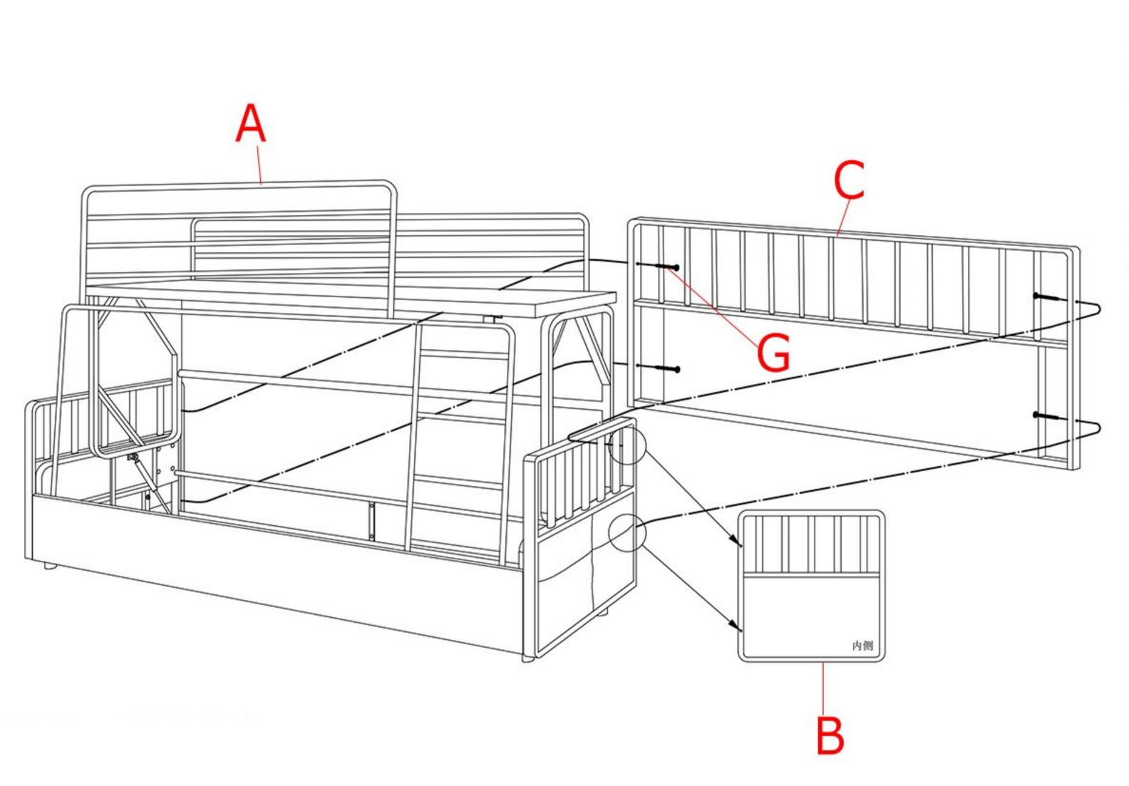
1. Screw up the side cushion frames (B) with the bunk bed body (A) with 4 small screws (E) on each side as shown in the picture.
