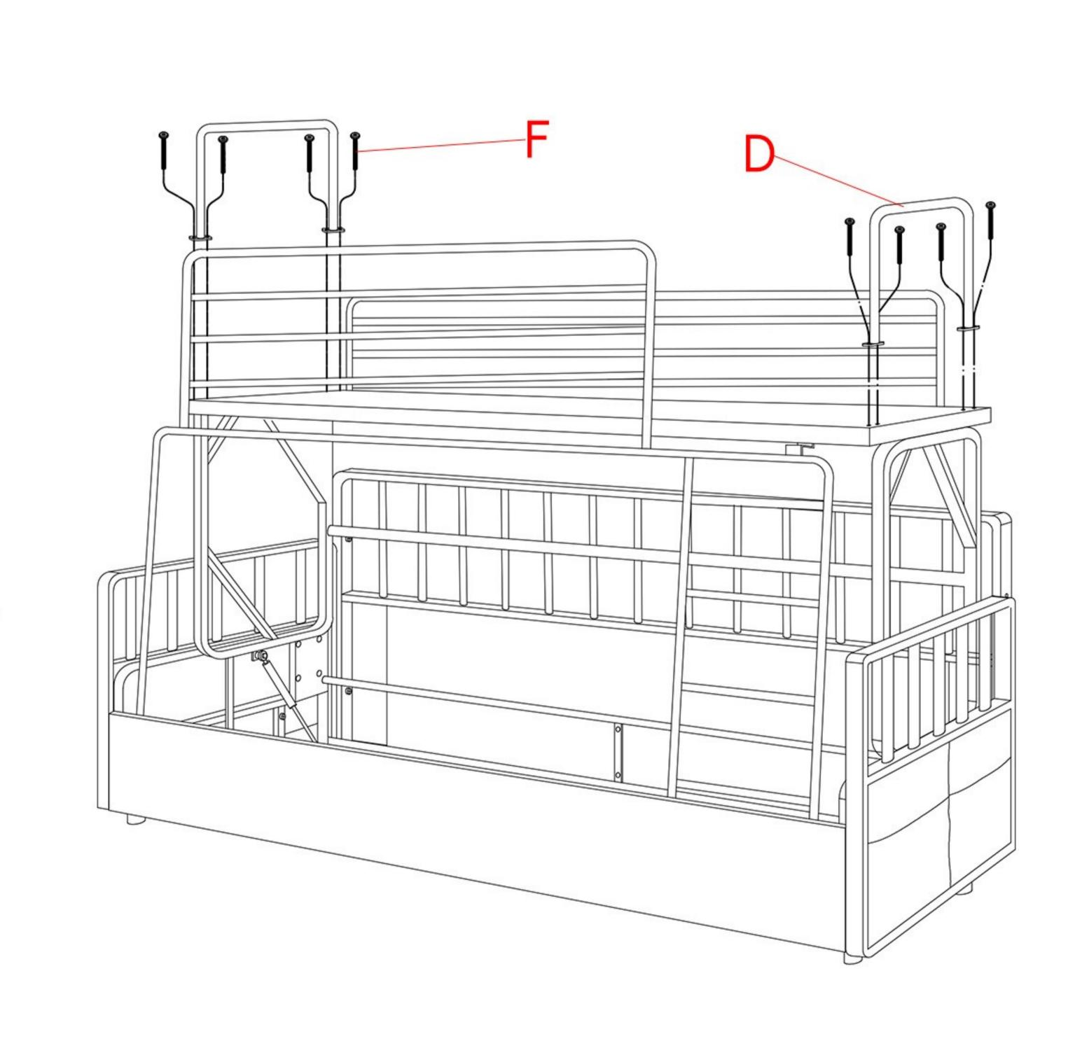
3. Install the N-shape frames (D) to each sied of upper bed by screwing 4 medium screws (F).
