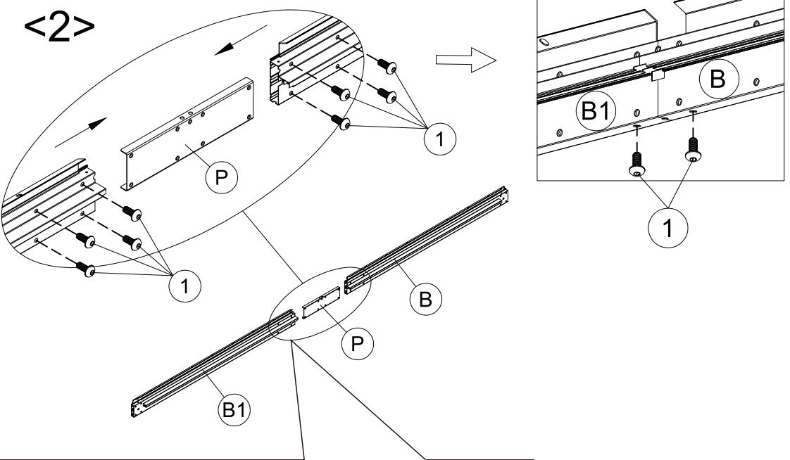
EN: This is divided into up and down directions, and the position of the hole refers to the enlarged view.
