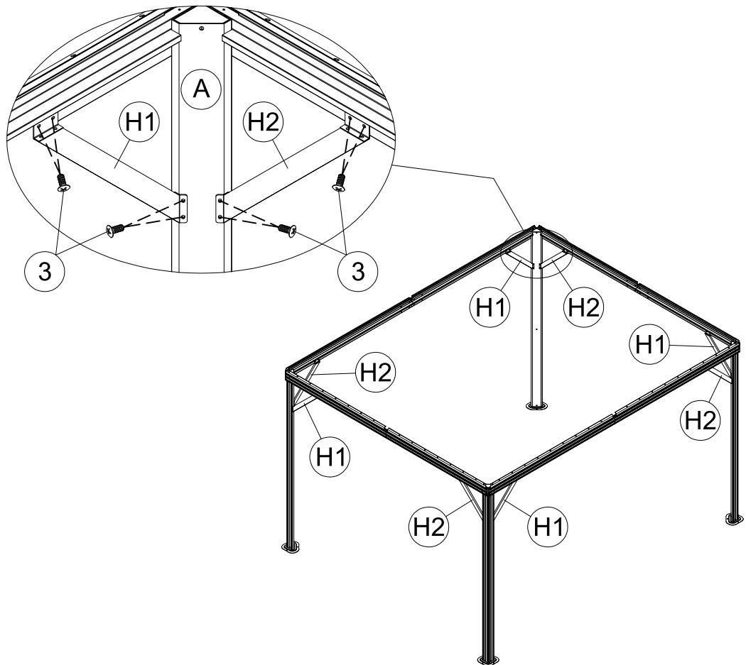
EN: Firstly, Install the screws on the beam, but do not tighten them. After the uprights are tightened, then tighten the screws all. If the hole position is not aligned, move the uprights to adjust the position.
