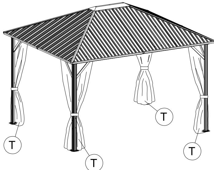
EN: 1.S and T are divided into left and right directions, identification method: take apart the four zippers, and install S/T in a single piece.
