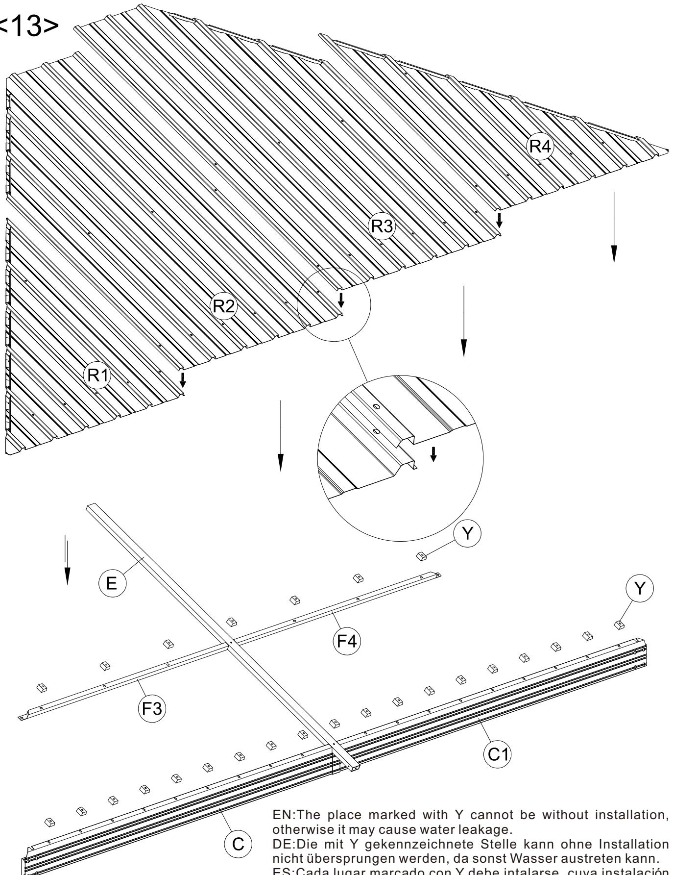
EN:The place marked with Y cannot be without installation, otherwise it may cause water leakage.
