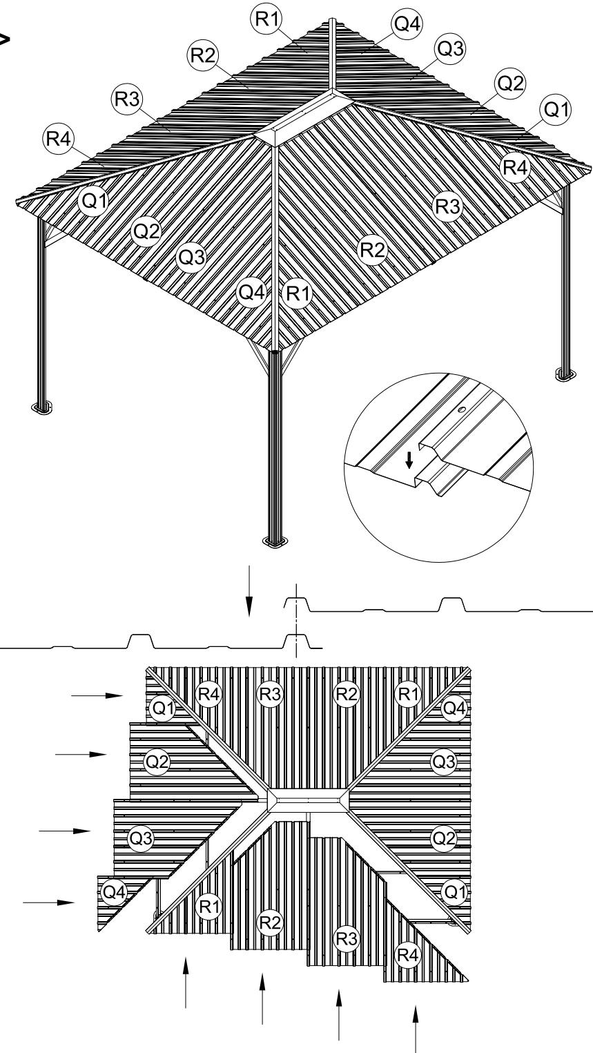
EN: This letter does not indicate the installation steps, just a schematic diagram of the iron plate distribution. The iron plate must be installed from left to right, not from right to left.
