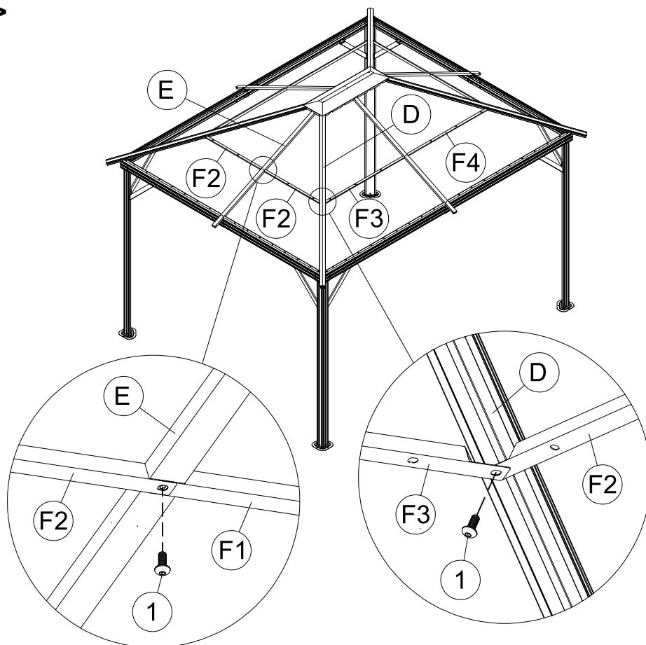
EN: Install in the same direction, do not tighten screws fully until all parts are connected.
