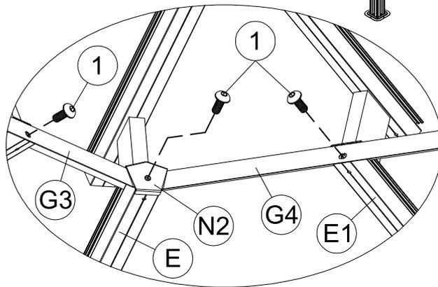
EN: Install in the same direction, do not tighten screws fully until all parts are connected.
