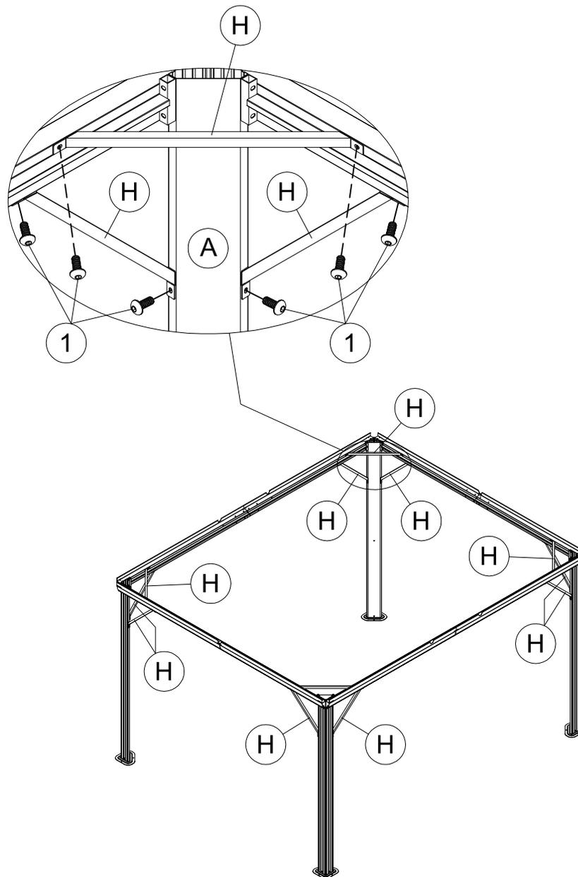
EN:Firstly, Install the screws on the beam, but do not tighten them. After the uprights are tightened, then tighten the screws all. If the hole position is not aligned, move the uprights to adjust the position.
