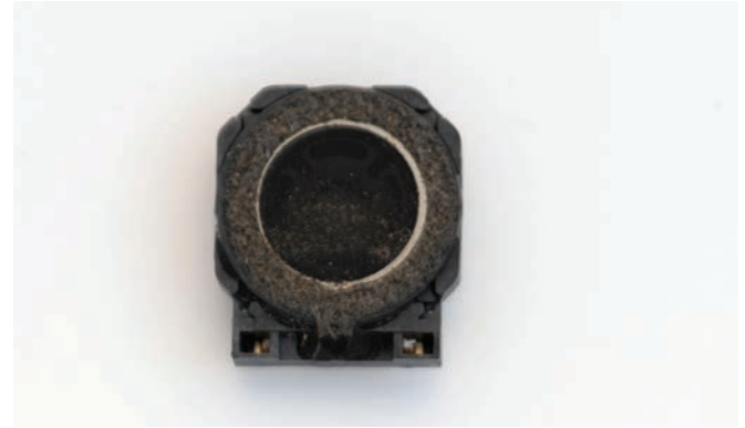
5 Cell phone speakers can be an option. The iPhone 8+ speaker (left) is 49.4mm x 18mm x 3mm with its upper right tab trimmed off. The Samsung S5 speaker (right) measures 17mm x 15.1mm x 4.4mm.
