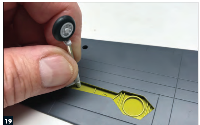
19 The fit of the outriggers to the wing is poor. I had to cut down the "pin" and shave off the tip of the triangular aft support to get each strut to fit into the opening in the wing.
