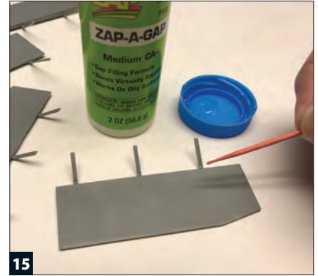
15 The suspension arms molded to the dropped flaps are very thin and break off easily. I reinforced them with a drop of gap-filling superglue applied where they meet the flap.
