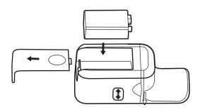
Open the compartment as in the diagram.
