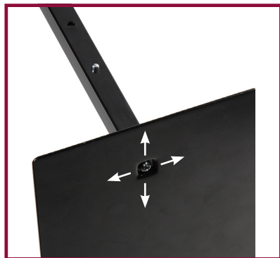
Loosen screw to remove arm and rotate in 90° positions. Adjust height with push button.
