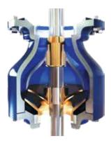
Optional construction features include bowl and impeller wear rings for extended impeller life. Keyed impellers for ease of disassembly and thrust balancing to put less strain on the driver assembly.
