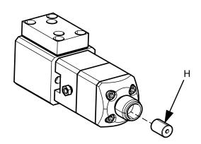
1. To minimize dead space in dispense valve 243666, place (H) in nozzle before attaching MOLSA Head.
