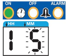
This confirms that the second digit for ON TIME is being configured in Minutes (MM).
