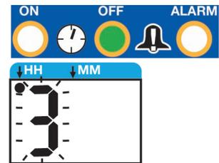
This confirms that the controller is ready for the first digit to be configured for OFF TIME in Hours (HH).
