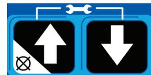
The first digit on the display begins to blink. This indicates SETUP MODE. After entering SETUP Mode, if no activity is detected, after 60 seconds a timeout occurs and the controller resumes in RUN MODE.
