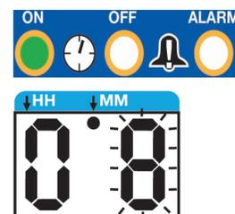
This confirms that the second digit for ON TIME is being configured in Minutes (MM).
