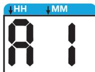
After entering ADVANCED PROGRAMMING, if no activity is detected for 60 seconds, a timeout occurs and the controller resumes RUN MODE.
