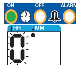
This confirms that the controller is ready for the first digit to be configured for ON TIME in Minutes (MM).
