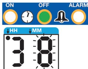
This confirms that the second digit for OFF TIME is being configured in Hours (HH).
