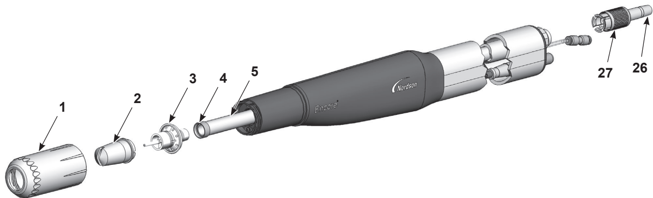
Figure 16 Powder Wear Parts Replacement
