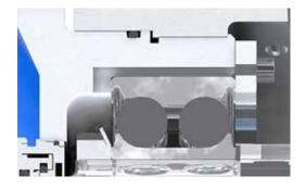
Double Row Angular Contact outboard and single row, deep roll inboard bearings provide excellent axial and radial load support.
