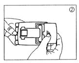
Note: Your unit will not function if the batteries are inserted incorrectly. To check, press the (1) button once and the LCD display will start up. Having made this check press the () button again to switch the unit off.
