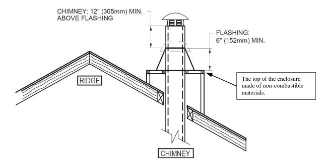
Note: The chimney chase on the roof must be the same size as the flashing.
