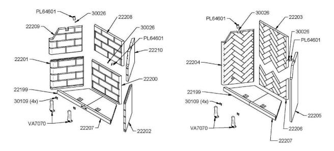
Figure 38 - Replacing FP11 Frontenac refractory panels
