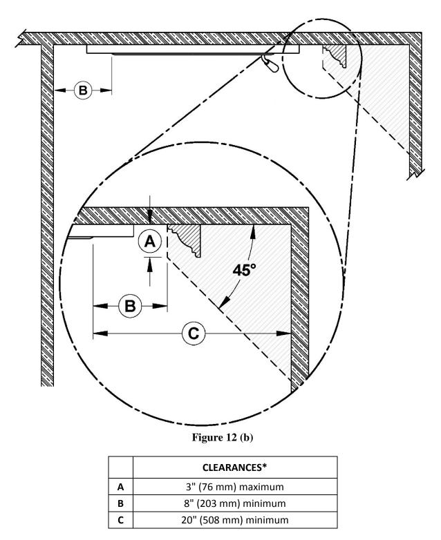
\*The fireplace can be installed against one of the walls in the room, respecting minimum value (B) from door opening. If the fireplace has a wall built against one side of the fireplace, the other sidewall must respect minimum value (C) from door opening. The fireplace may also have a combustible side mantle respecting values (A) and (B).
