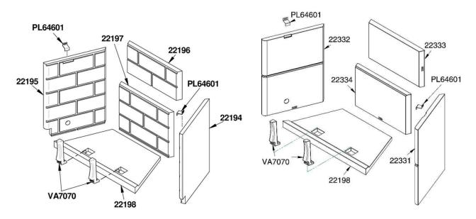
Figure 41: Replacing Antoinette refractory panels
