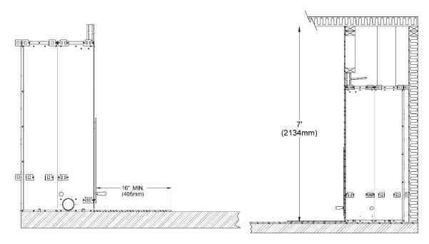
Figure 8 Installation on raised base
