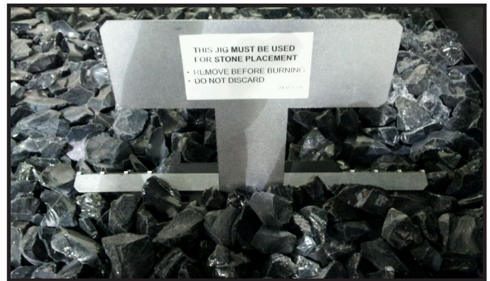
Figure 9.9 Rock Placement Jig
