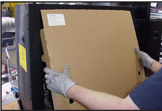
Figure 11.5 Installation of Splatter Guard
