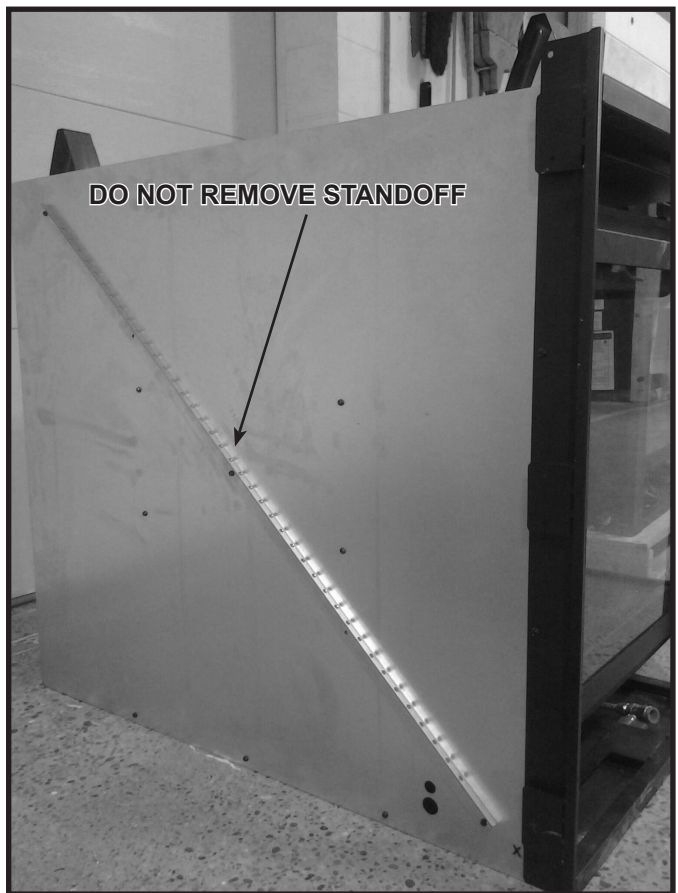
Figure 2.3 Do Not Remove Standoff
