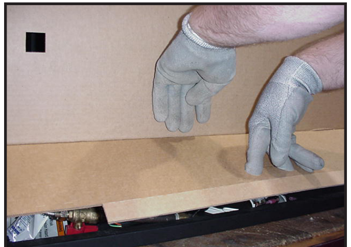
Figure 11.9 Opening Lower Access Panel
