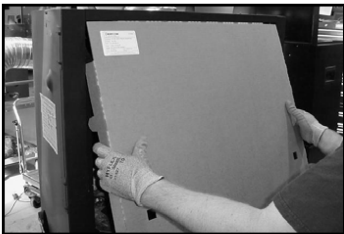
Figure 11.5 Installation of Splatter Guard
