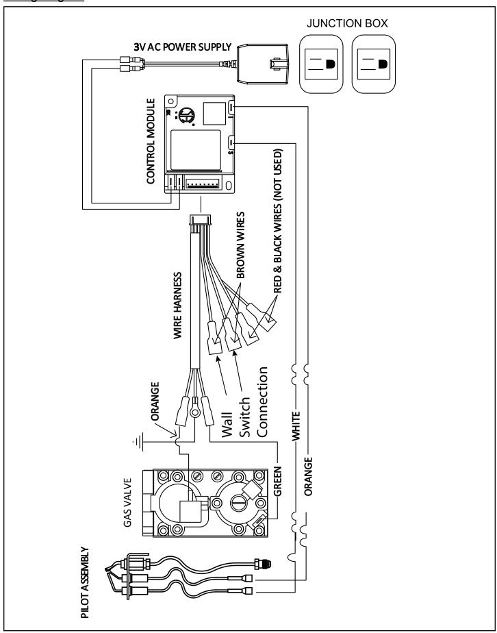
Figure 5.2. Wiring diagram
