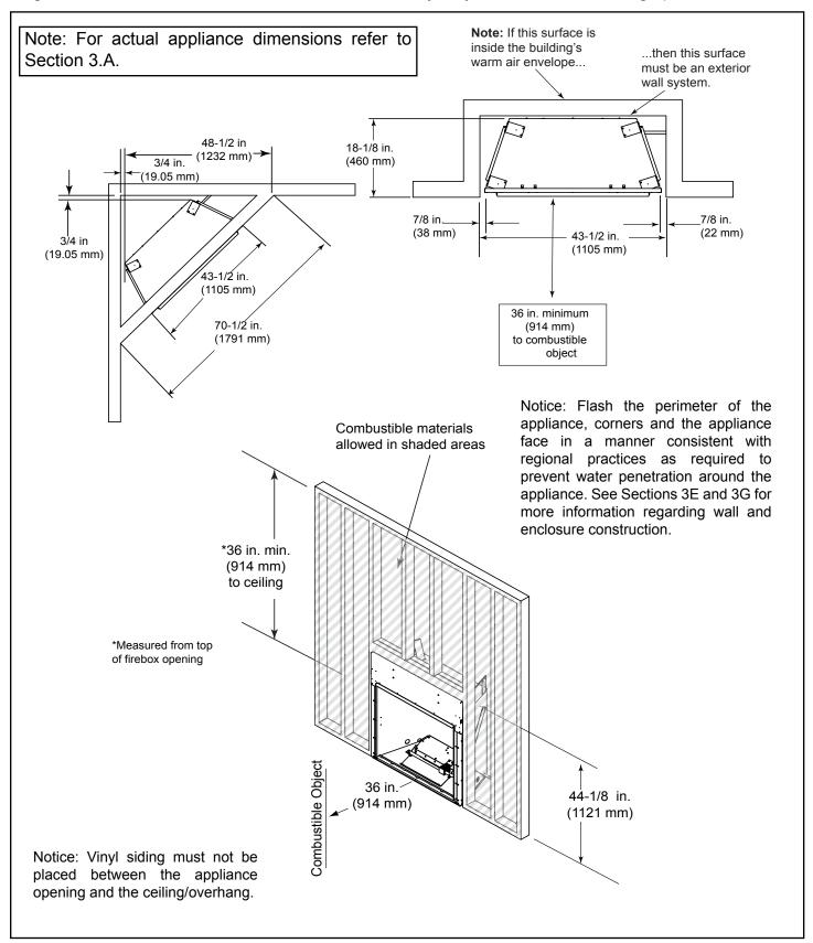
Figure 3.1. Appliance Locations and Framing Dimensions - ODCOUG-36
