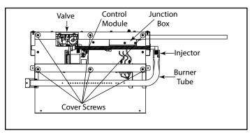
Figure 6.1. Engine Assembly
