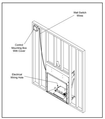
Figure 3.6. Wall switch mounting
