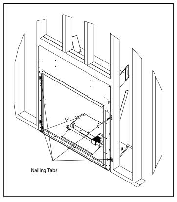
Figure 4.1. Positioning and Securing Nailing Tab
