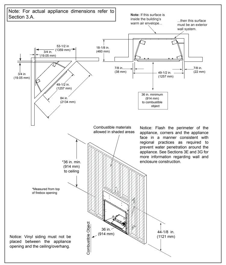
Figure 3.2. Appliance Locations and Framing Dimensions - ODCOUG-42
