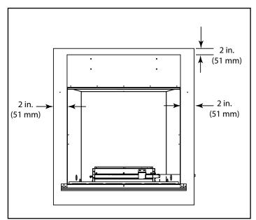
Figure 3.7. Front View Tape Location
