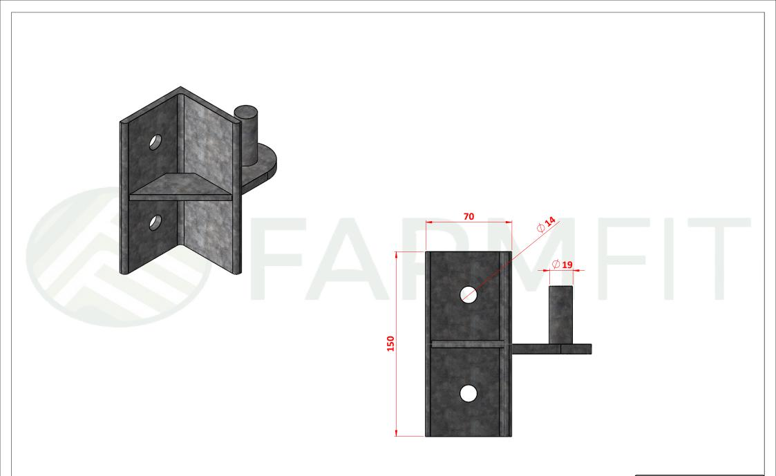
Gates, Cubicles, Yokes, Feed Barriers, Sheep Equipment, Handling Systems, Concrete Products, Water Products, Posts, Fixings, Bespoke Fittings, Roofing, Ventilation & Much More! HINGE ON RIGHT HAND ANGLE (SINGLE)
