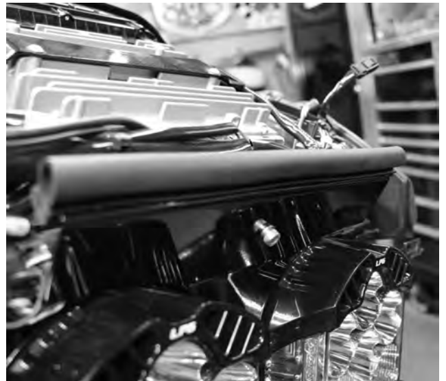
Bulb Seal Slides On to Top of Shield
