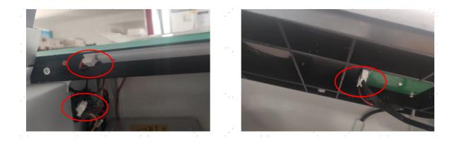
Remove the front and rear screws and remove the panels. Replace them using the same screws and then restore the electrical connections.
