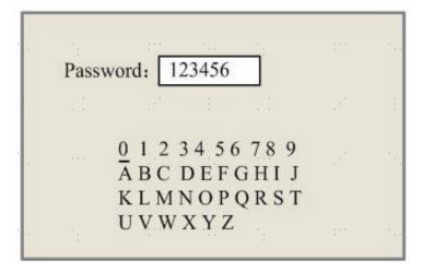
Push ← or → and ▲ or ▼ to select a password and press ENTER to save it. The current parameters of the machine will be stored as its defaults. They can then be retrieved by using the Restore Default Parameters command. It is recommended that you save your machine's actual factory default settings, so they can be easily restored when need be.
