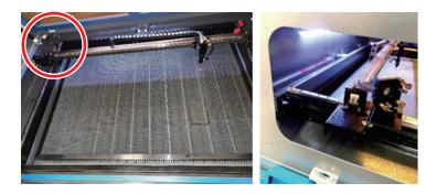
Once set, place a piece of tape on the 2nd mirror's frame. **DO NOT** place the tape directly onto the mirror. Repeat the steps from §5.4.1. If the laser is not centred on the 2nd mirror, you will need to adjust the 1st mirror's set screws accordingly.
