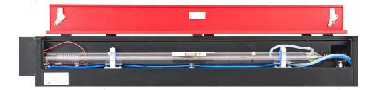
You will need to place a piece of tape at each stage of the laser path, marking it to confirm that that stage remains correctly aligned. When it is not, you will use the laser tube's brackets or the screws on the back of the misaligned mirror to correct the problem. Once the provided tape runs out, we recommend masking tape as it is easy to manage and use.
