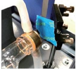
**DO NOT** place the tape directly onto the mirror. Turn on the machine and set the power level to 15% or lower.
