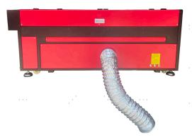
The other end should be connected to a dedicated purifier or (if the fumes are not hazardous and meet local and national air safety standards) placed out a window. **NEVER** operate the laser if the vent is not purifying or removing the fumes produced by the target material. Research materials before use and never operate the laser on any (such as PVC, teflon, and other halogen-containing substances) that can produce corrosive, hazardous, or even deadly fumes.
