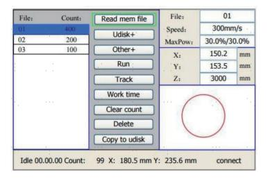
The system will automatically read the memory files. The file name and the work times will be listed and the selected file will be previewed in the upper right corner. Different memory files can be selected by using ▲ or ▼. Press ENTER to preview the selected file on the main interface. Press ESC to close the preview.
