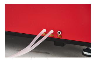
Connect the water pump to its power supply. For best results, use a power outlet on a separate fuse from the engraver itself. If no such outlet is available, the pump can also be plugged into a dedicated socket located on the side of the engraving cabinet. Once the pump is plugged in, water should begin to run through your machine and back into your tank. **ALWAYS** obtain visual confirmation that the water is flowing through the laser tube before starting your laser.
