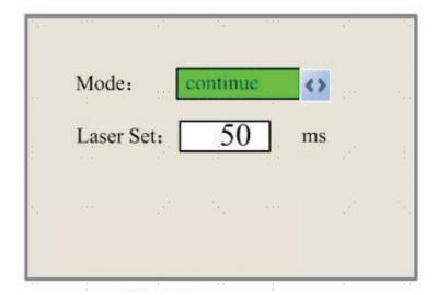
The operation method is the same as the previous setting. When Continue is selected, press **PULSE** to fire the laser, and release the key to finish firing. When Manual is selected, pushing **PULSE** will fire the laser for precisely the period shown beside Laser Set in this screen.
