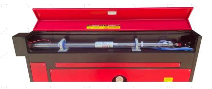
Step 4. Inside the main bay, remove the nylon cable ties from the X axis and the honeycomb table.
