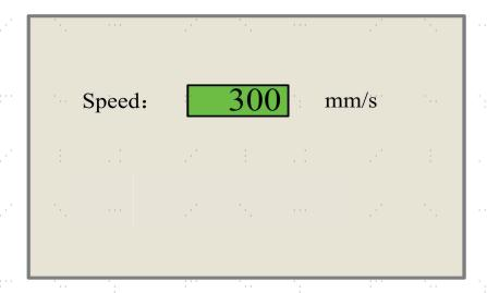
A cursor will appear when pushing  $\blacktriangleleft$  or  $\Rightarrow$ . Move the cursor to the numeral area and push  $\blacktriangle$  or  $\blacktriangledown$  to change the value. Press **ENTER** to save the change. Press **ESC** to invalidate the change and return to the main interface.
