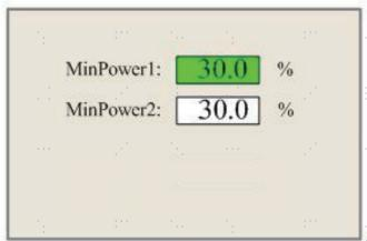
When  $\mathbb{Z}/\mathbb{U}$  is pushed, the green block can move up and down to denote the changing item. Then  $\triangle$  or  $\nabla$  and  $\leftarrow$  or  $\Rightarrow$  can be used to change the value. Press **ENTER** to save the change. Press **ESC** to invalidate the change and return to the main interface.
