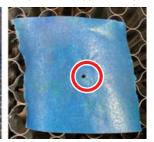
When the laser is well centred along the entire path from the tube to the workbed, your laser mirrors are all correctly calibrated and (assuming they are clean) performing at optimum efficiency.
