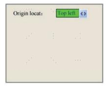
This interface sets the relative position of the origin. Different origin positions can generate different reflections of the graph over the X/Y axis. The operation method is the same as those described above.
