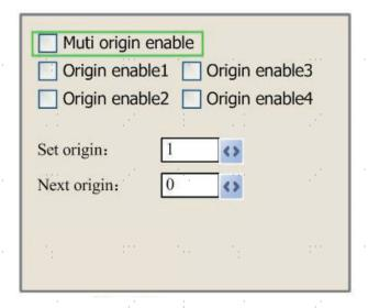
Press **Z**/U to select an item. When Multi Origin Enable is selected, press **ENTER** to enable or disable the item. When enabled, the small box will be red and, when disabled, the small box will be grey. When selecting Set Origin or Next Origin, push • or • to select the value. When changing the parameters of Set Origin, remember to press **ENTER** to validate the change. Parameters will be saved automatically when the interface is closed.
