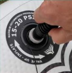
4. Pump board to pressure between 15-20psi
