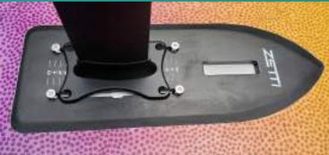
6. Move screws through the slots and into the countersunk recession on the mast base
