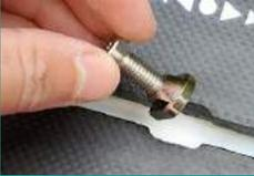
4. Insert T-nut assembly into US Box (2 each) and move to all 4 corners of track
