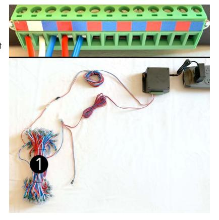
**Step 5:** Attach the input end of the second LED string to the output end of the first LED string. Attach the power injection wires at the output end of the second LED string to the controller box.
