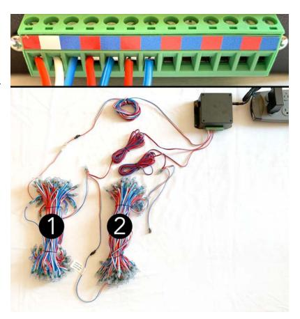
**Step 6:** Attach the input end of the third LED string to the output end of the second LED string. Attach the power injection wires at the output end of the third LED string to the controller box.
