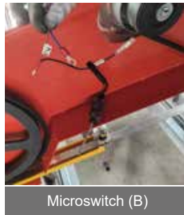
Step. 3: Find the Emergency Stop Switch(A) and the Microswitch (B)
