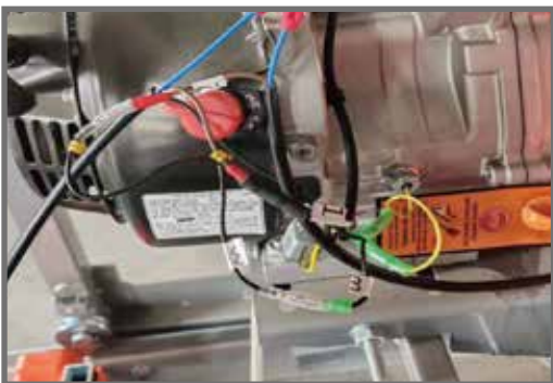
Step.5: Connect the A1 and 1 (Female) Connect the B3 and 3 (Male)
