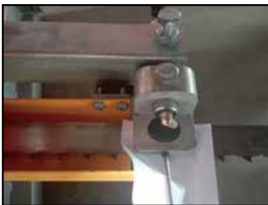
Adjusting the gap above the saw blade
