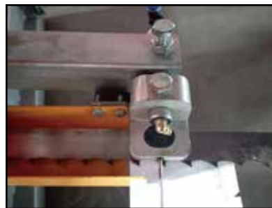
Adjust the gap below the saw blade
