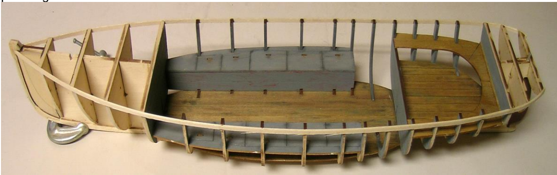
Photo 2: the completed hull structure ready for planking
