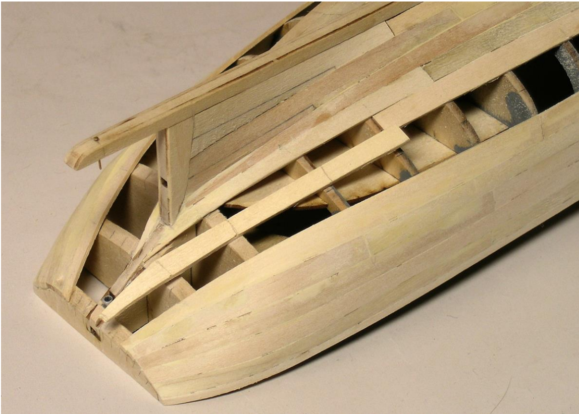
Photo 7: The shape of planks at the stern
