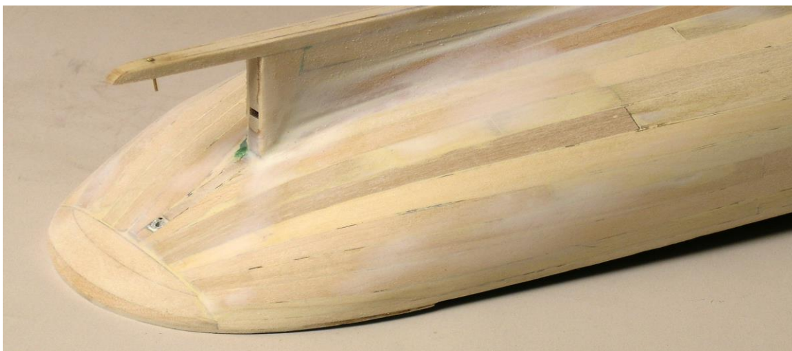
Photo 8: The completed fantail stern. Sanding and filling has begun
