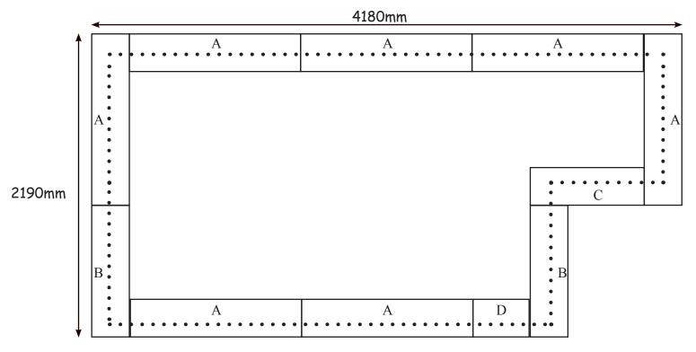
Sleeper Lengths: A = 1220mm (48") B = 970mm (38") C = 860mm (33") D = 360mm (14")
