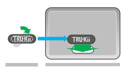
Align locking Press TRU·Kii oval firmly into oval hole in tray clamp arm with TRU-Kii oval from top side of tray.
