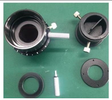
Clean the prism with an air blower or use the cotton bar soaked with alcohol. Please make sure the prism is free of any damage.
