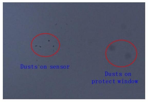
The dark spot on the right is the shadow of dust on the protective glass. The very small black spot on the left is the shadow of dust on the chip. In the above situation, it is recommended to blow off the dust on the glass surface with air. The remaining dust is recommended to be removed with calibration flat frames.
