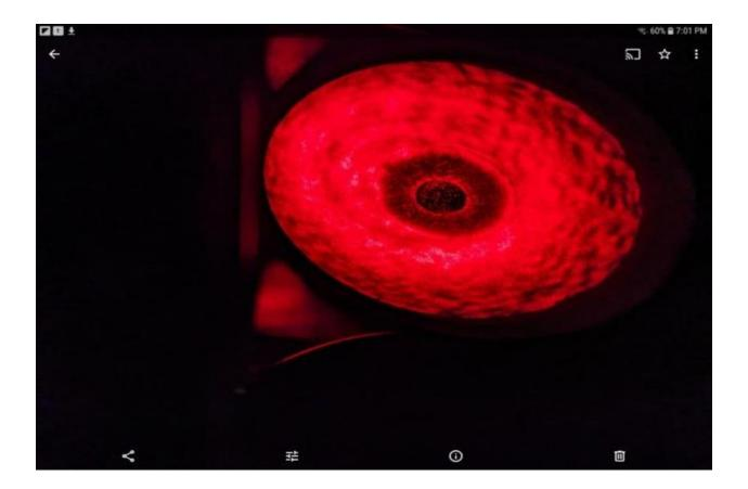
\*\*If the center marker is of a certain size, there will be a small red circle of light outside the central hole of the TuBlug screen and inside the shadow of the primary's center marker. You can use this as an aid to collimation by making that small illuminated ring perfectly uniform in thickness.
