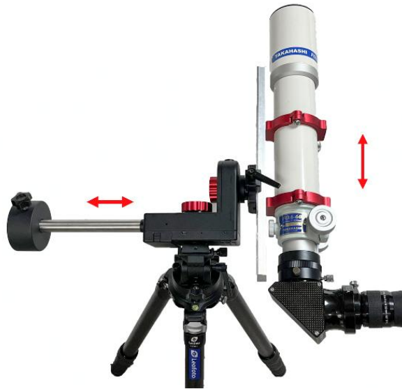
Figure 13 Balancing a telescope
