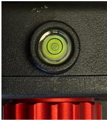
Figure 17 Leveling a SkyHunter in AA mode
