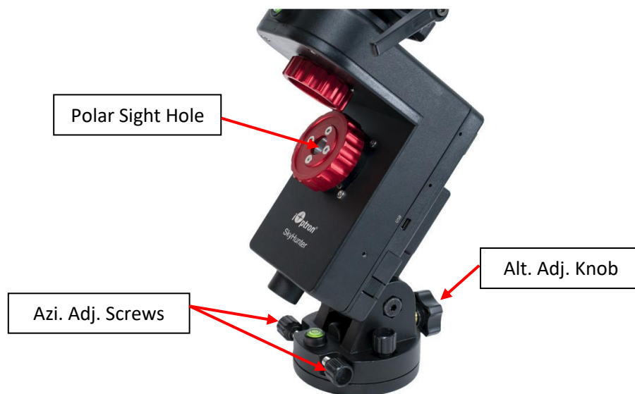
Figure 15 Polar alignment through Polar Sight Hole
