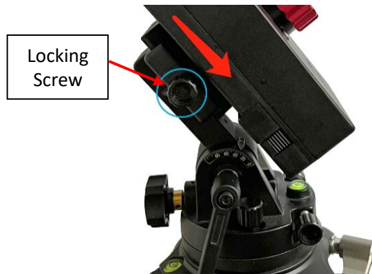
Figure 9 Slide mount head into an EQ base
