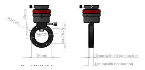
The samples that connect with all kinds of front part. Connect with M42/0.75 to 2inch adapter (made by QHYCCD)
