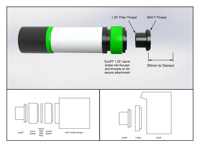
Using a DSLR and T-ring is simple since the backfocus is then a standard 55mm. Many mirrorless cameras also have longer T-rings that provide a 55mm distance. For using an astronomical CMOS camera, you will need spacers to achieve the required 55mm. The ZWO cooled cameras, for example, include the necessary 16.5mm and 21mm spacers. For other cameras you may need optional spacers. Please contact if you have questions on setting up the correct backfocus.
