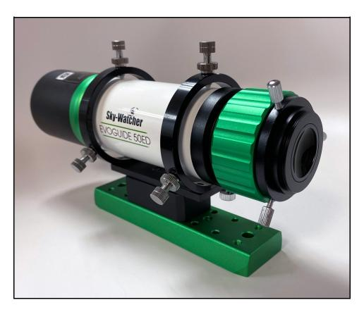
Add the camera and any necessary spacers and you are ready to go! The focuser will be most of the way in toward the telescope when using the EvoFF, so you may have to thread the green helical focuser ring clockwise (as viewed from the camera end) most of the way to reach focus. The helical is surprisingly fine and makes focusing for imaging very easy. If you have used a similar mechanism on a camera lens you will be pleasantly surprised how much easier it is to use the EvoGuide focuser.
