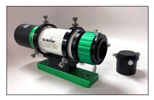
Be sure the three thumb screws are backed out far enough that they do not interfere with sliding the 1.25" barrel into the focuser. Then insert the EvoFF into the focuser and thread in into place. (There is often a little push back from the air in the tube, so don't be surprised at that.) You can then tighten the three thumbs screws for added security. Just don't forget to loosen them before removing the EvoFF!
