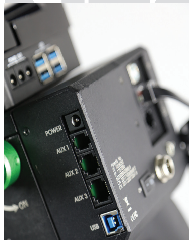
Cable management features four USB 3.0 ports, three 2.1mm power ports and three serial ports
