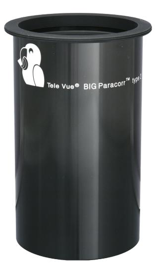
**Big Paracorr type 2** Newtonian coma corrector • 3" O.D. • 15% magnification factor • removeable top flange 3.40"-24 threads • 80mm Back Focus • Prime Focus moves 72.3mm out from native focus position • Weight: 24 oz. • Length to base of flange: 5.1"
