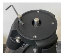
Step 2: Add the bottom half of extension onto the tripod top. Insert two M6 screws to secure the bottom half on to the tripod top.
