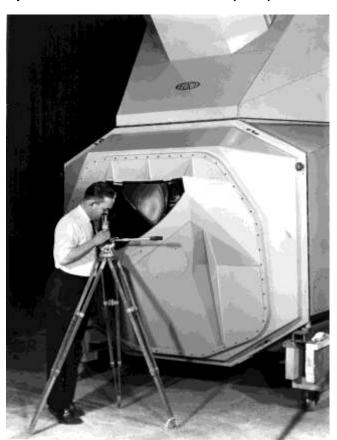
Seen at left is one of the Infinity Display Projectors that fit over the LEM simulator. A separate unit was required for each window of the spacecraft. You can see why the astronauts affectionately dubbed the full collection of simulators for the Apollo mission "The Great Train Wreck!"
